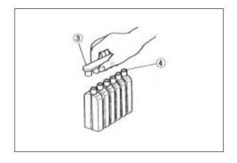
Insert the nozzles of the electrolyte container into the battery's electrolyte filler holes, holding the container firmly so that it does not fall.
