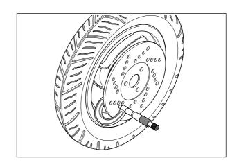
• With the disc mounted on the wheel, check the disc for face runout with a dial gauge as shown. Replace the disc if the runout exceeds the service limit.
