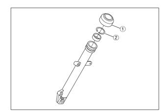
Remove the oil seal by using the special tool.
