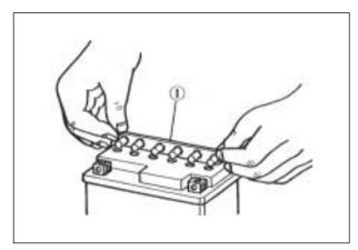
Using the pocket tester, measure the battery voltage.
