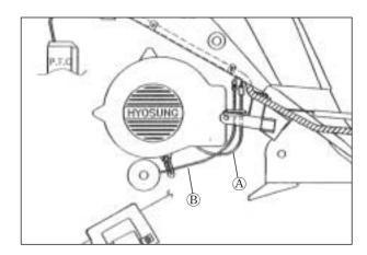
After remounting the engine, route the wiring harness properly and following adjustments are necessary.
