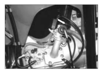
• Install the air vent hose ①, oil hose ② and fuel hose ③.
