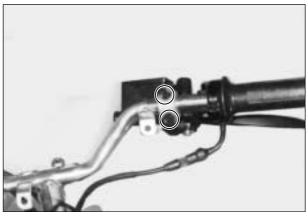
■ Remove the brake lever ① and brake switch ②.
