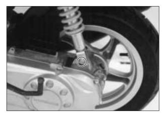
Remove the engine mounting shaft and remove the engine from the frame.
