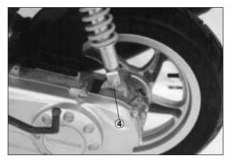
■ Install the magneto lead wire
