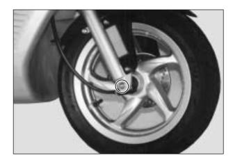
• Remove the disc plate ① by removing the bolts.
