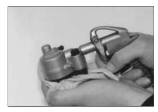
● Remove the dust seal ① and piston seal ②.
