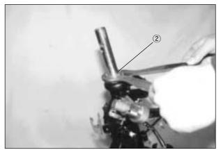
● Install the handlebar and tighten the set bolt ① and clamp bolt ② to the specified torque.
