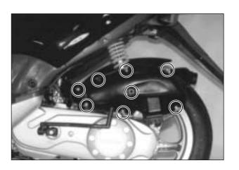
Remove the air cleaner cover, separate the element.
