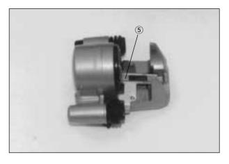
Place a rag over the piston to prevent popping up. Force out the piston with a air gun.
