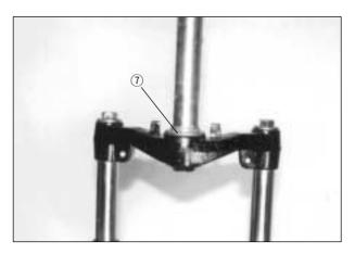
• Remove the steering stem steel balls ①.
