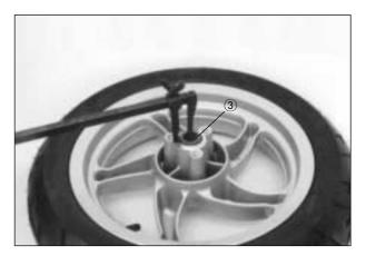
Drive out the both bearing with the special tool in the following procedures.
