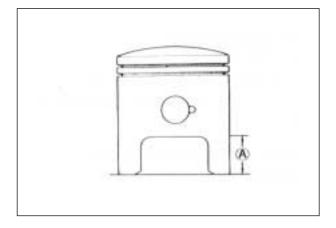
As a result of the above measurement, if the piston-tocylinder clearance exceeds the following limit, overhaul the cylinder and use an oversize piston, or replace both cylinder and piston. The measurement for the bore diameter should be taken in the intake-to-exhaust port direction and at 20mm from the cylinder top surface.
