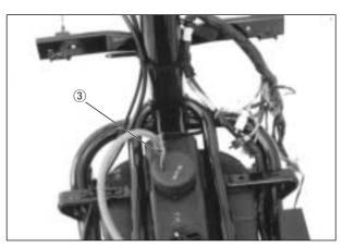
• Remove the six fuel tank mounting bolt.
