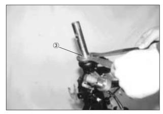
Remove the front fork assembly by removing the lock washer 4, steering outer upper race 5 and dust seal 6.
