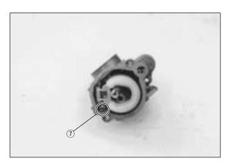
• Install the thermoelement assembly.
