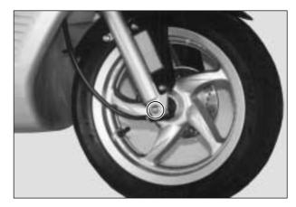
Tighten the caliper mounting bolts to the specified torque.
