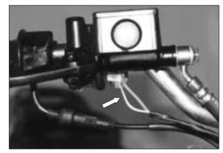
Place a cloth underneath the union bolt on the master cylinder to catch spilled drops of brake fluid. Unscrew the union bolt and disconnect the brake hose/master cylinder joint.
