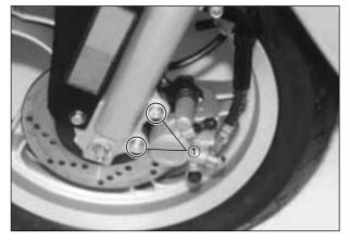
• Reassemble it after remove the brake pads ①.
