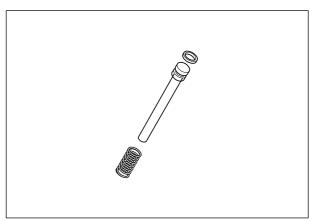
● Inspect fork pipe and bottom case sliding surfaces for any scuffing or flaws.
